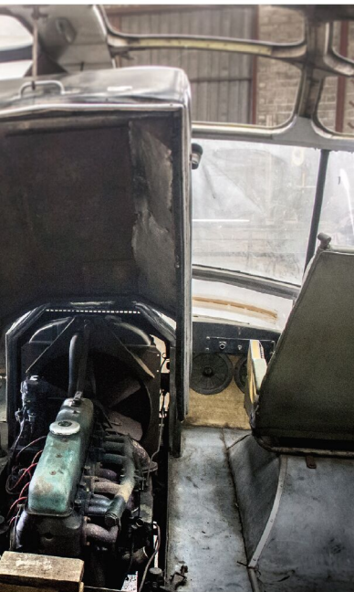
Six-cylinder petrol engine is capable of 90 hp. Original gauges are still intact.
