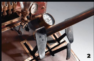
2 Clutch is on the left, brake is on the right, and the gas pedal is in the middle.
